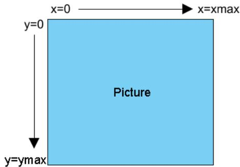
Where **xmax** is the x-size of a full size image (1279 pixels), and **ymax** is the y-size of a full size image (1023 pixels).
