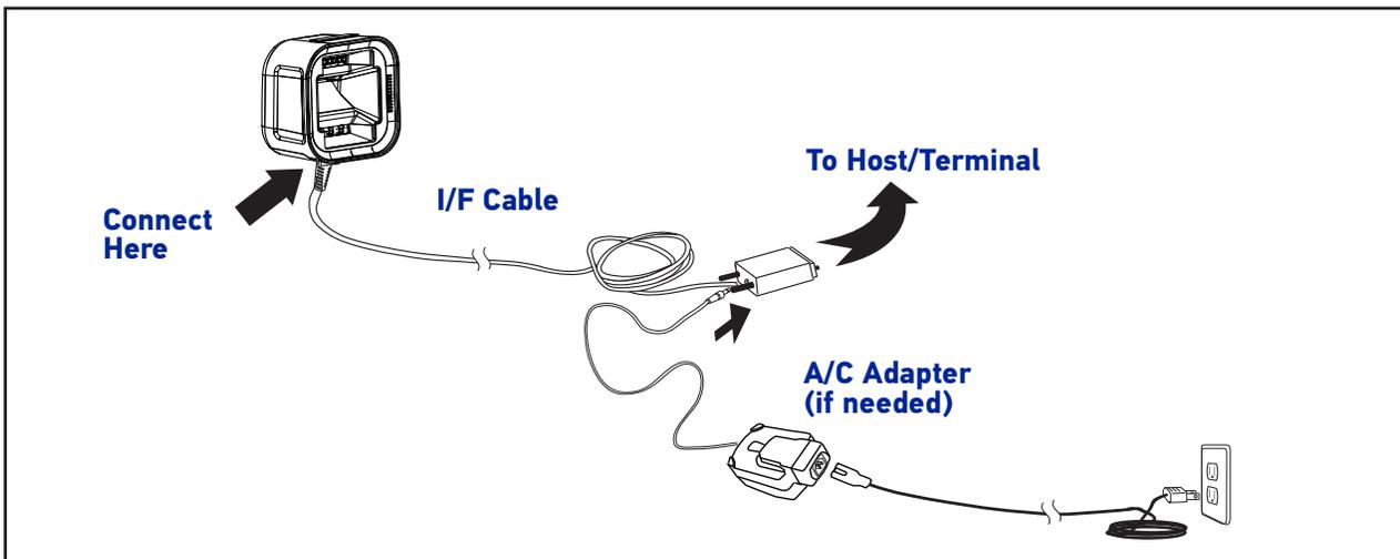
**USB Connection :** Connect the scanner to a USB port on the terminal/PC using the correct USB cable for the interface type you ordered.
