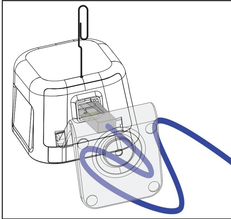
2. If the EAS cable is present, free it from the notch in the bottom cover before pulling the Stand away from the unit, as shown on [page 7](#).
